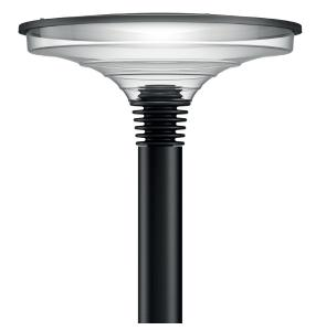
**BECCO** is born with LED and many necessary components are integrated parts of the luminaire design. The heat sink forms a characteristic connection between the column or bollard and the lantern, and it is the base of the LED module as well. The light source is not visible, and the indirect, non-glaring light is spread by means of the arched roof plate.
