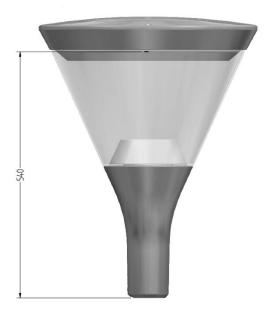
Typing the light centre height, you will see that the mounting height is wrong. However, this will not influence your calculation. If the pole height is 4 metres, you shall type the light centre height as 4.0 m + 540 mm = 4.540 m.
